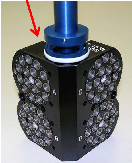
4 uni-pucks inserted into adaptor cassette
