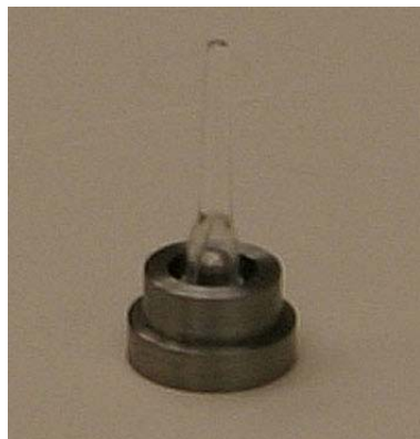
Figure 2. Image of a plastic capillary mounted a magnetic pin.
