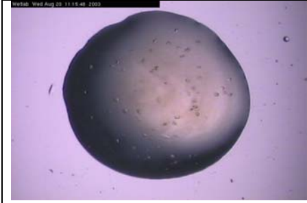
Figure 18: TSCP with dTMP crystals in a hanging drop. The solution is tinted yellow due to the presence of the protein..
