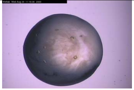
Figure 19: TSCP with dTMP crystals in a hanging drop. Gel Precipitate has formed in the solution.
