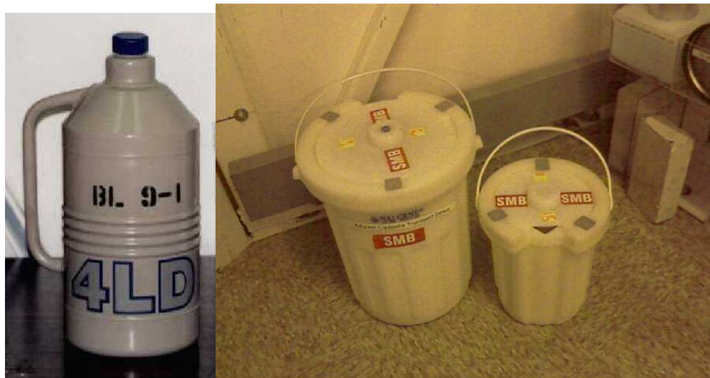
Figure 3: Dewars available at the beamline. The two white Nalgene dewars can be used for short term cassette, pucks or samples storage and transport; the 4LD dewar can be used for dispensing liquid nitrogen.
