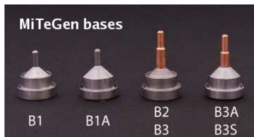
Figure 10: Commonly available pin types
