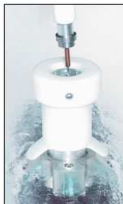
Figure 21: a. Placing the guide tool into the cassette. b. Putting the pin on magnet tool. c. Picking the crystal.
