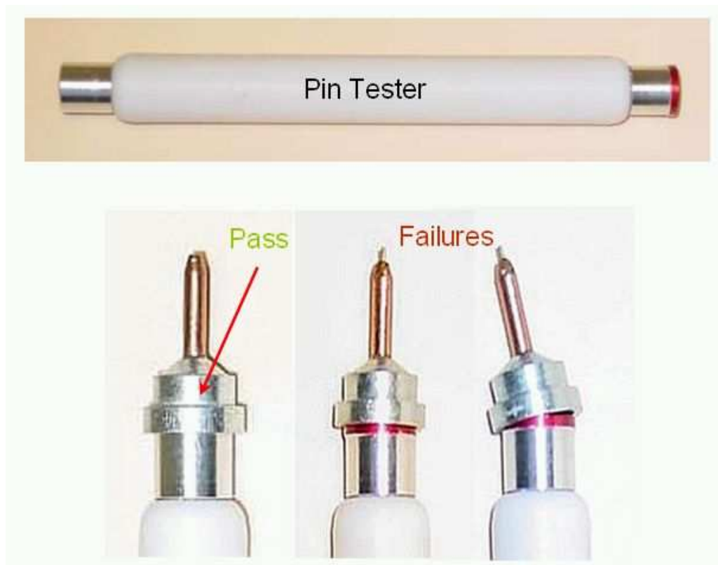
Figure 13: Use this tool (included with the SAM kit) to test all your pins before use with the SAM robot
