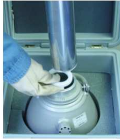
Figure 25: Placing the Teflon support ring (C) inside the shipping dewar
