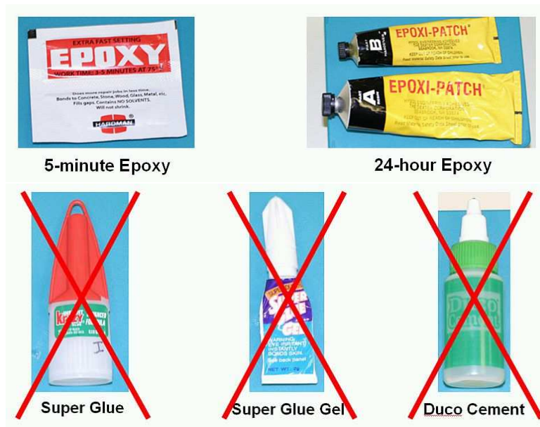
Figure 12: Use Epoxy to affix the microtubes to the sample pins. Glues other than Epoxy have been observed to cause sample mounting errors.
