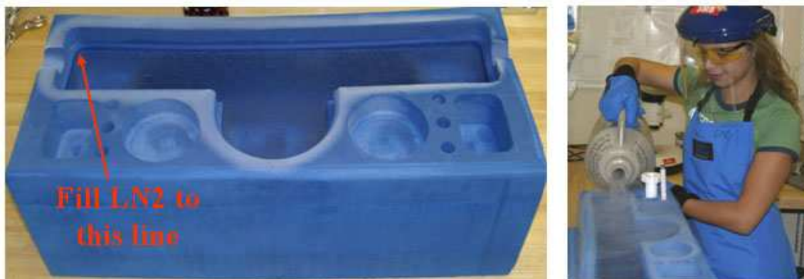
Figure 19: Filling the custom foam dewar
