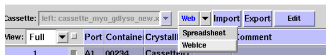
Figure 33: Launching a web browser window running Web-Ice from the Blu-Ice screening tab.
