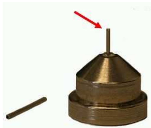
Figure 11: Broken microtubes used with Magnetic pins can make the pin jam inside the cassette port, stopping the robot.
