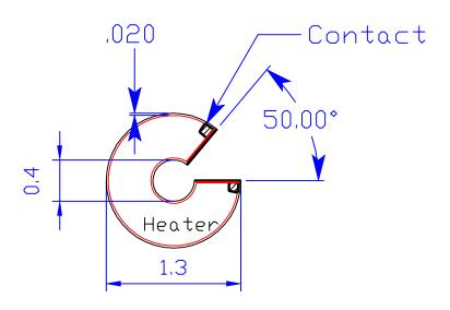
Printed-circuit flexible heating element on a substrate of a capton film attached to 0.3 mm thick Al foil. Should be wrapped into a cone and glued into the heat shield using a thermoconductive compound (Eccobond 285 or similar).
