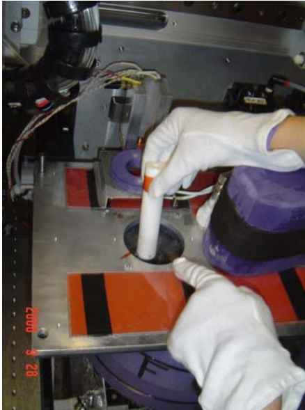
Fig. 7 Inserting puck lid into the dewar
