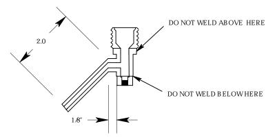
DRILL HOLE IN SIDE AND WELD 1/8" SS TUBING TO THE SIDE.
