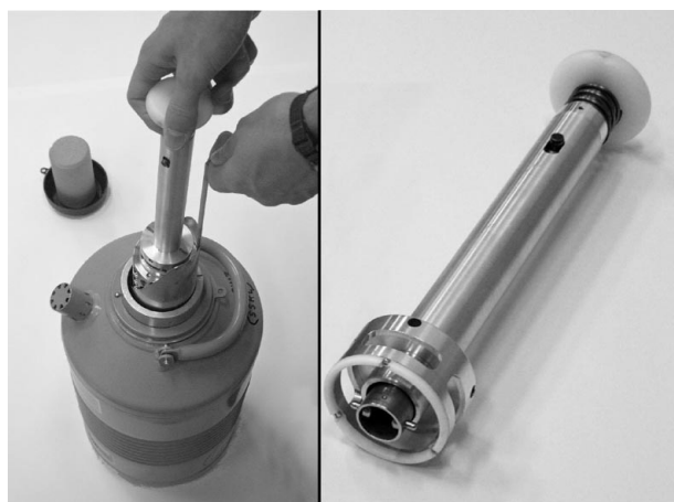
Figure 5 Unloading a sample cassette from a Taylor Wharton CP100 shipping Dewar using the manual transfer handle.
